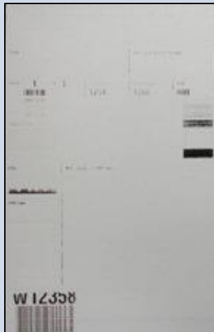
Shipping label printed with an under charged battery (Figure 3)
